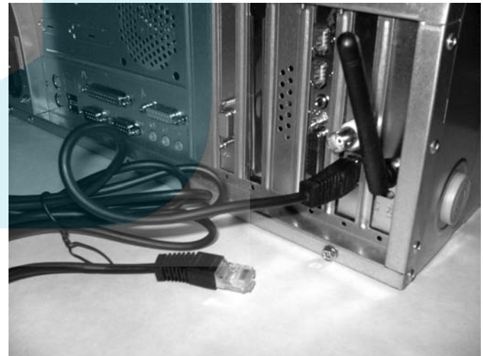
Figure 16-2: The bridging computer should have both Ethernet and Wi-Fi adapters.
